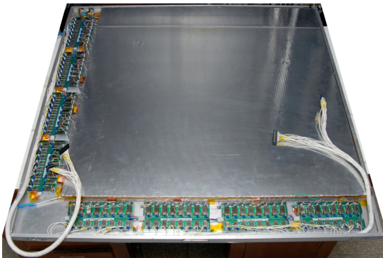
Fully assembled large area glass RPC (1 m \times 1 m)
