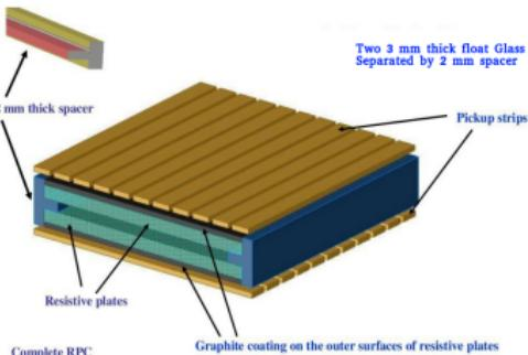
Resistive plate chamber (RPC) (active element) sandwiched between iron plates (passive element)
