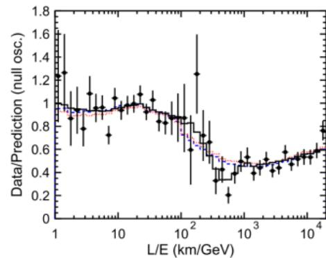
The Super-K experiment was the first experiment to confirm the sinusoidal  $L/E$  dependence of the  $\nu_\mu$  survival probability by observing a dip around  $L/E = 500 \text{ km/GeV}$ .
