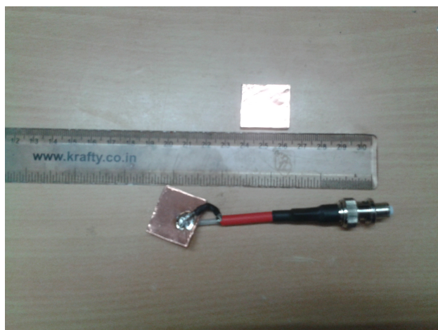
Figure 3.13: The copper tape electrode on the surface of glass.
