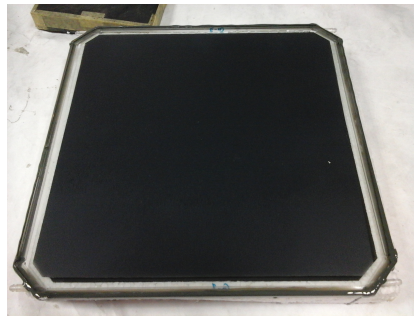
Figure 3.7: RPC after applying glue to the Edge Spacer
