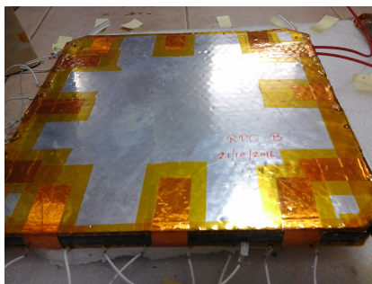
Figure 3.12: RPC after packing in pickup panels
